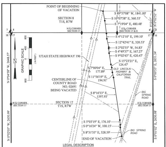
An existing road in the SW ¼ SE ¼ of Section 8 and the E ½ of Section 17, all in T1S, R7W, S.L.B.&M., Tooele County, Utah, the centerline of said existing road being more particularly described as follows:
