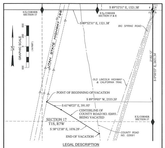
An existing road in the SW ¼ NE ¼ and the N ½ SE ¼ of Section 17, T1S, R7W, S.L.B.&M., Tooele County, Utah, the centerline of said existing road being more particularly described as follows.
